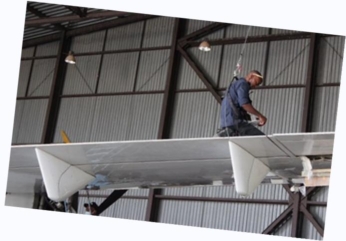
b) Using safety harnesses on elevated platforms
