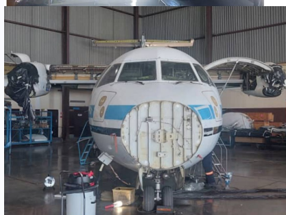
e) Both nose and tail sections are also stripped down for corrosion inspection ►
