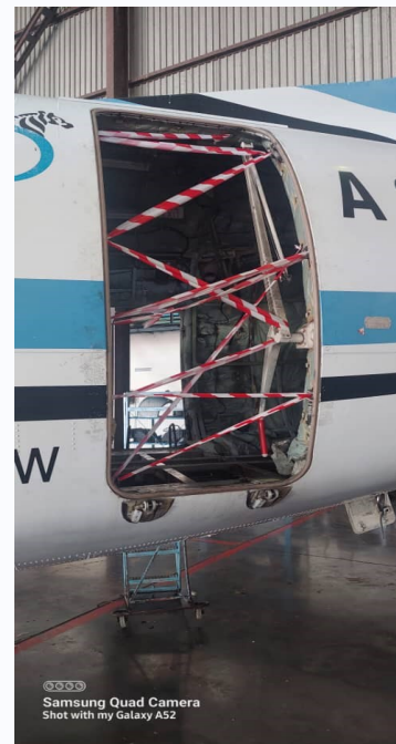
d) Proper cordoning is in place to ensure no unauthorized access during maintenance ▲
