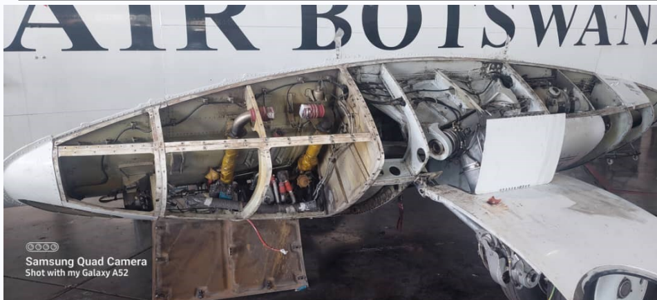
a) Aerodynamics fairing panels opened for corrosion inspection ▲
